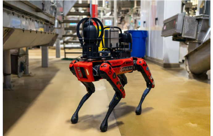
Nestlé Purina incorporated Spot into its maintenance routine to automate thermal and acoustic inspections on the factory floor.
