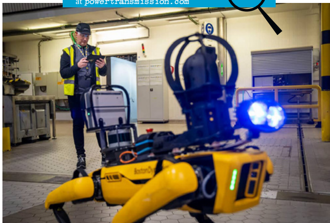
Spot conducts 1,800 individual inspections each week across ten packaging lines that churn out over 50,000 containers of beer at the Anheuser-Busch InBev in Leuven, Belgium.
