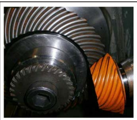
Figure 8 Pattern check after heat treatment and grinding to test seating features.
