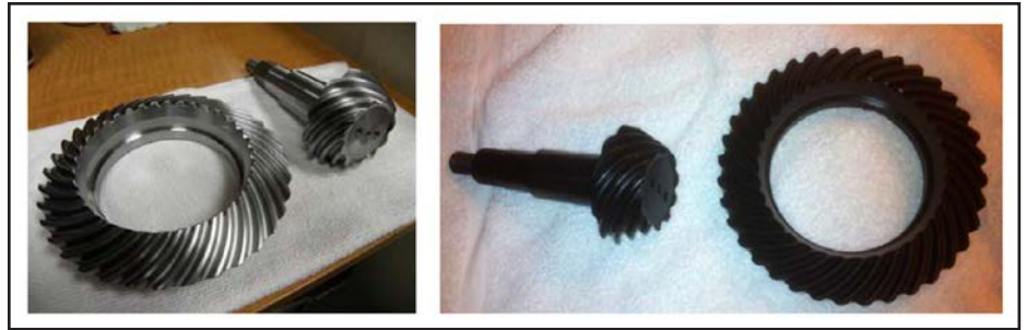
Figure 7 Ring and pinion prior to heat treatment, along with gears prior to installation.
