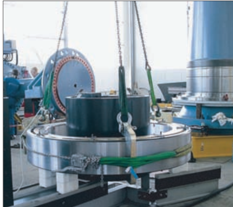
FIG. 4: Positioning the CARB® bearing system onto the custom-designed induction heater.
