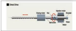
Figure 10—Drive mechanism of injection screw.
