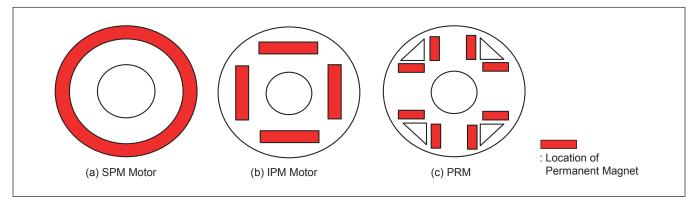
Figure 1—Rotor construction of permanent magnet motor.
