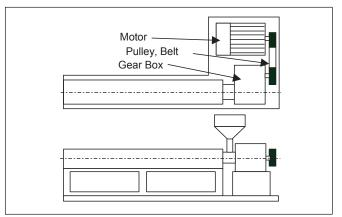
Figure 7—Belt and gearbox system.
