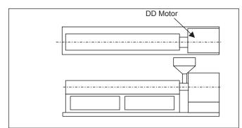
Figure 8—Direct drive system.
