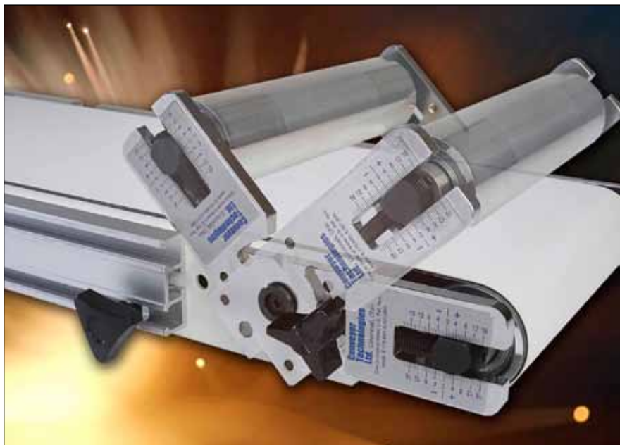
Figure 2—A tool-less, swing-up tail pulley provides one-minute belt exchange while retaining the tension setting. Calibrations on both sides permit rapid, precise balanced tension by which each increment represents the tension-setting-per-foot of conveyor length.
