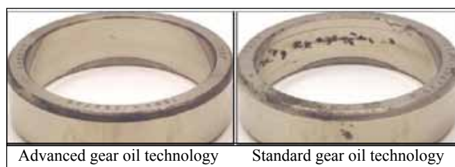
Figure 13—Emcor rust test with 0.5% NaCl water.
