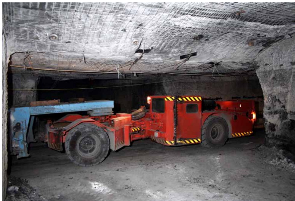
J.H. Fletcher's Prime Mover diesel tractor features a Mico electrohydraulic braking system.
