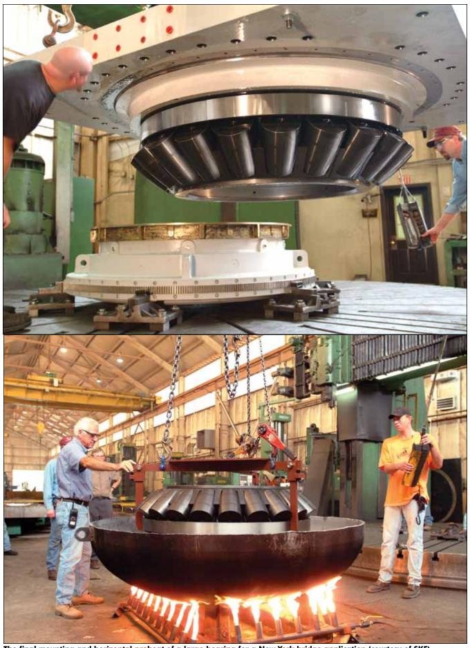
The final mounting and horizontal preheat of a large bearing for a New York bridge application (courtesy of SKF).
