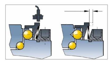
torque limiters. These can be used to limit torque as well as linear chain or belt pull. A torque limiter is essentially a mechanical circuit breaker. Rather than having a component that breaks and needs to be replaced, a torque limiter can trip and be reset many times during its life.
