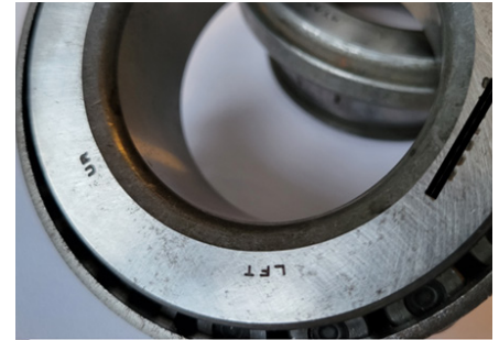
New Bearing: Dull surface, non-reflective, covered with grind lines
