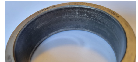
OBJECTIONABLE: Heavy thermal staining. Heavy wear lines.
