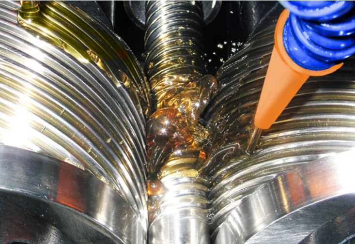
Figure 5 — Throughfeed lead screw rolling.
