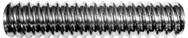
Figure 7 — Surface finish achieved by rolling operation.
