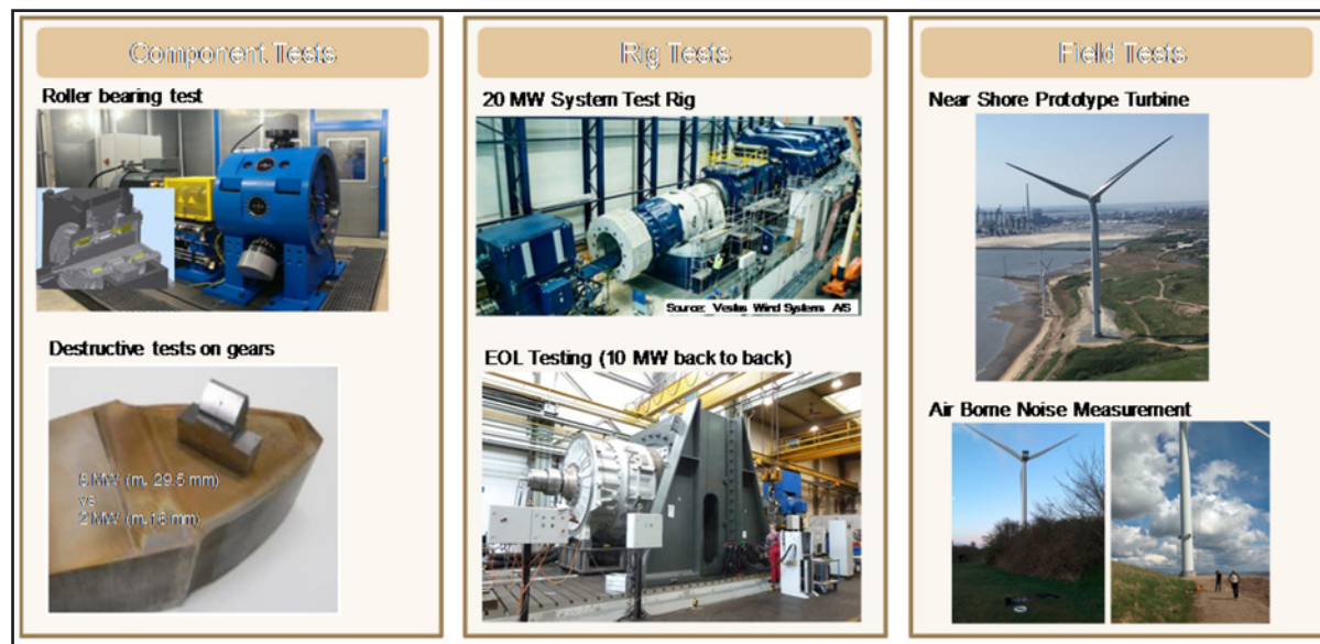
Figure 8 Validation procedure with component, system and field tests.
