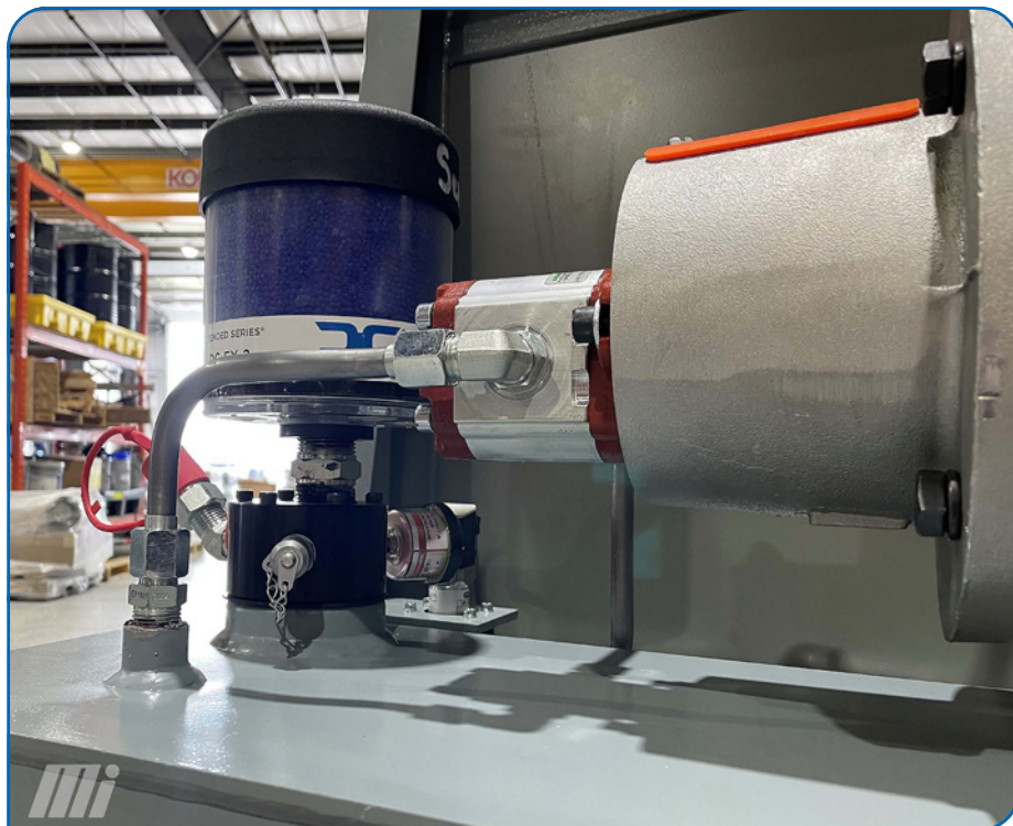
The sampling port (center view of the black adapter) is fed from a downtube that is positioned for samples to be taken from the working fluid, which is the optimal place. Image courtesy of Motion.
