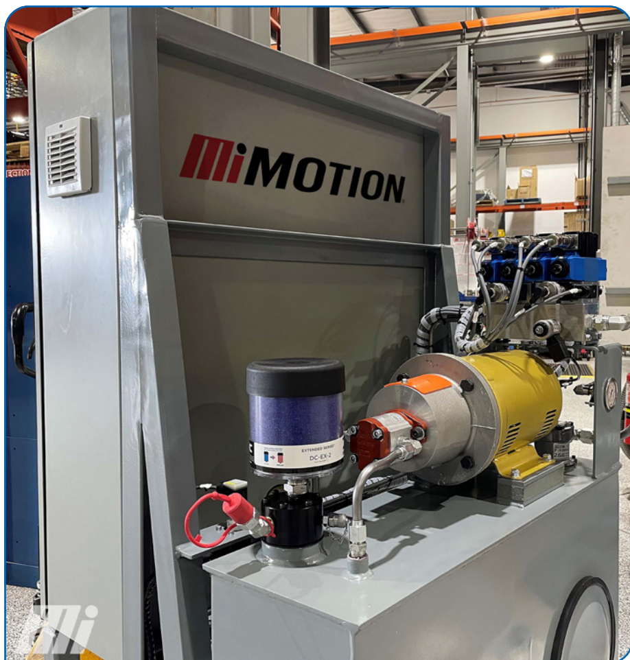
This hydraulic power unit is equipped with a clean fill/sample adapter. This adapter enables maintenance personnel to fill or sample the oil through a closed coupled connection. Image courtesy of Motion.
