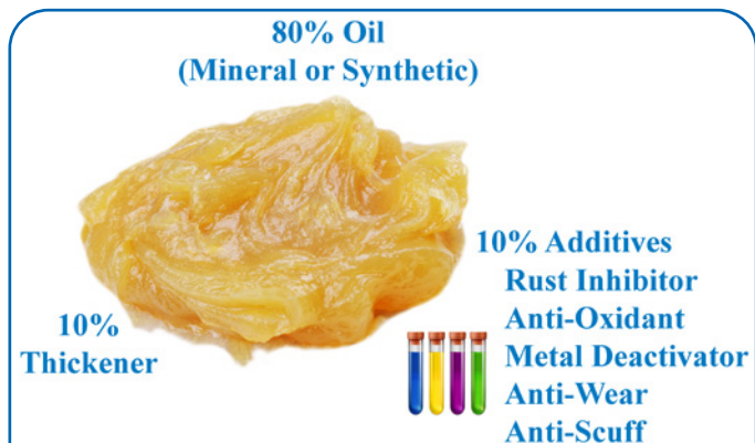
Figure 1 Diagram of grease composition (oil, thickener additive).
