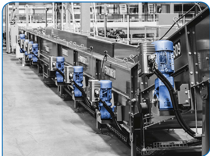
The larger an application, the more gearmotors it has, and the more its energy bills may be reduced through high-efficiency gearmotors. (Photo courtesy of Nord Gear Corp.)
