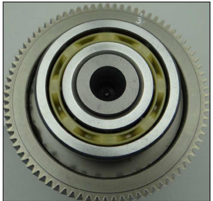
Figure 13 Sinter gear after torsional strength test.
