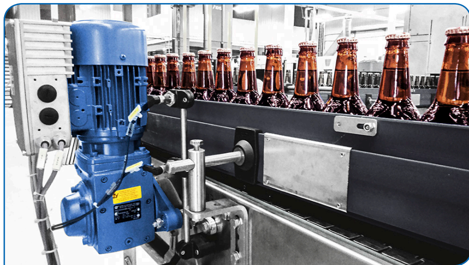
An application's load and speed, whether they're constant or variable, are considerations when trying to lower energy costs through high-efficiency gearmotors. (Photo courtesy of Nord Gear Corp.)
