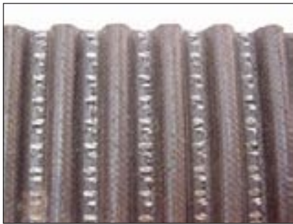
Figure 7—Excessive land area wear.
