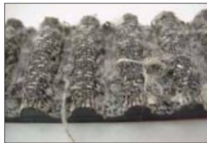
Figure 12—Extreme tooth wear from worn sprockets.
