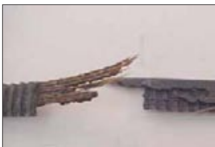
Figure 1—Normal fatigue failure.
