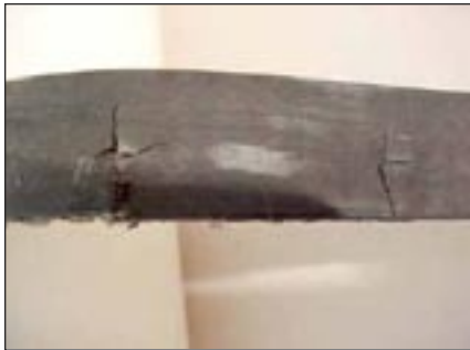
Figure 19—Tensile cord failure from debris.
