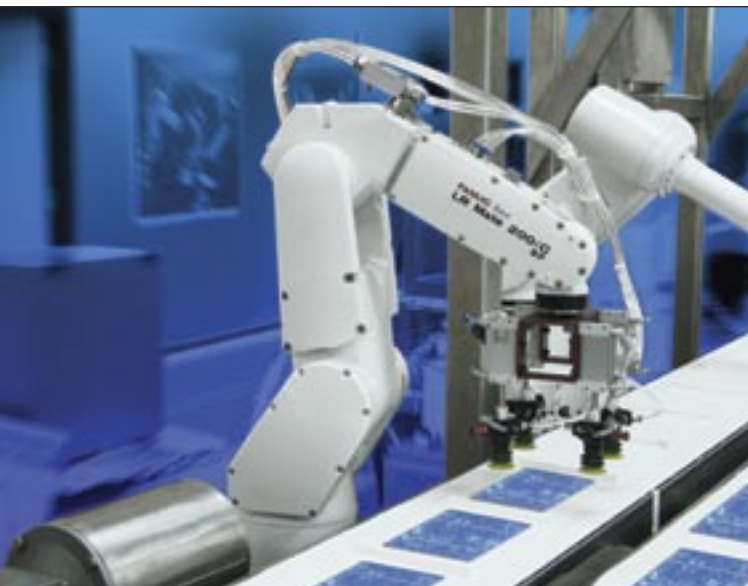
FANUC has incorporated vision, force control and accuracy tools into robotics used in solar manufacturing (courtesy of FANUC).
