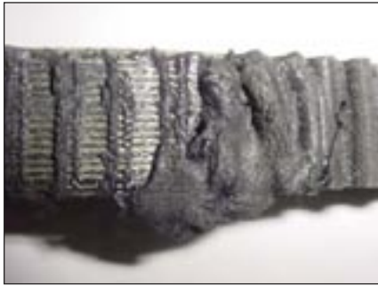
Figure 18—Melting from high-temperature operation, polyurethane.
