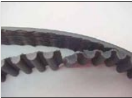
Figure 8—Tooth separation failure.
