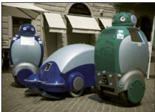
The DustBot project contains two robotic units, the DustClean and the DustCart, for street cleaning and waste removal projects (courtesy of Evelina Dario).
