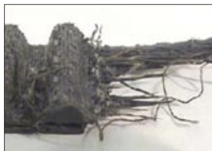
Figure 4—Typical shock load failure.
