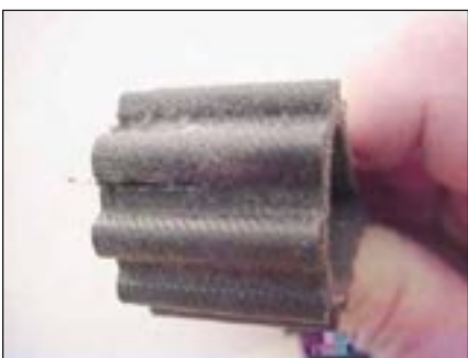
Figure 11—Uneven belt wear.
