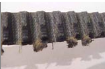
Figure 10—Extreme belt edge wear.
