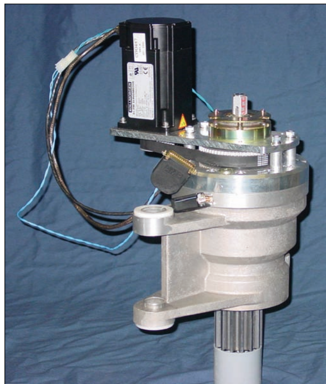
Figure 3—View of the azimuth drive unit removable module.
