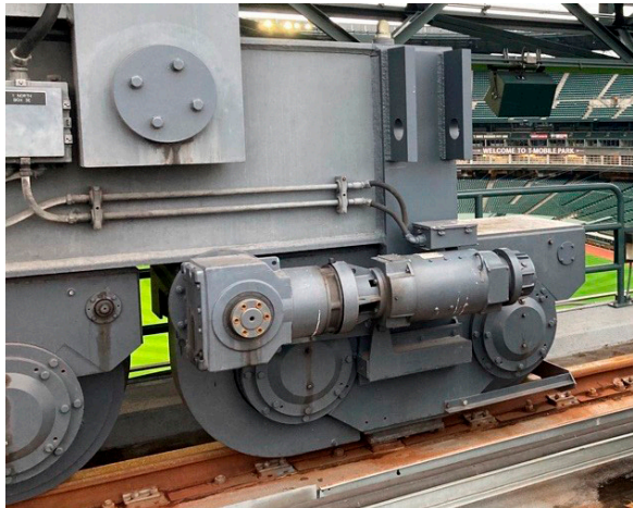
Figure 3—Retractable roof’s wheel drive.
