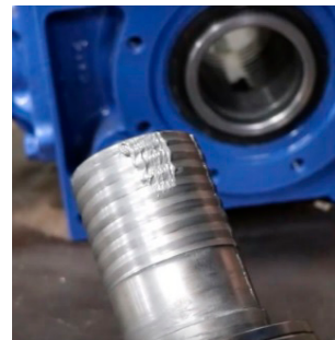
Figure 11 — Anti-seize paste used in a minimal surface area for Sumitomo’s Taper Grip Bushing.
