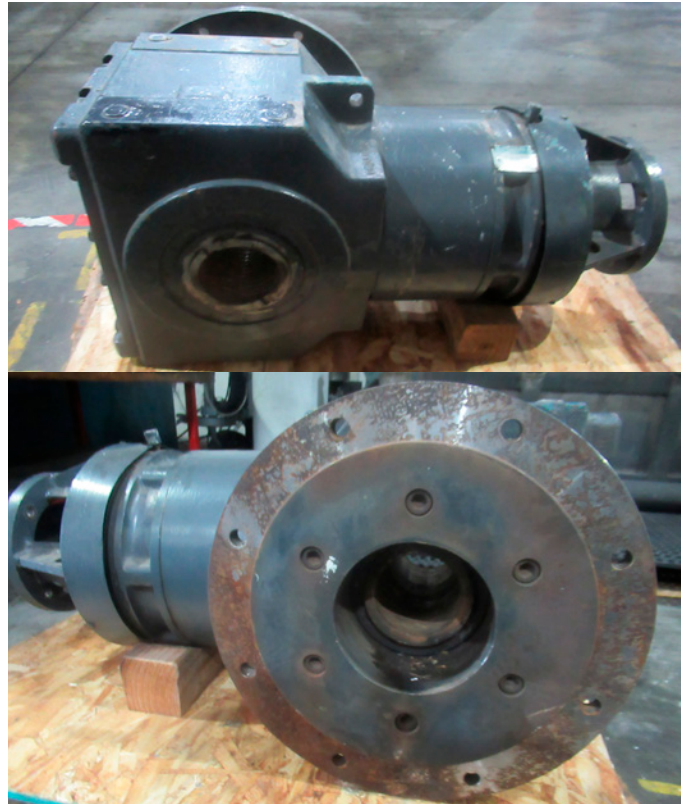
Figure 8—External condition of the gearbox. Back of the unit, no defects (top). Front of the unit, leakage on low-speed shaft seal and mild rust on the mounting surface (bottom).
