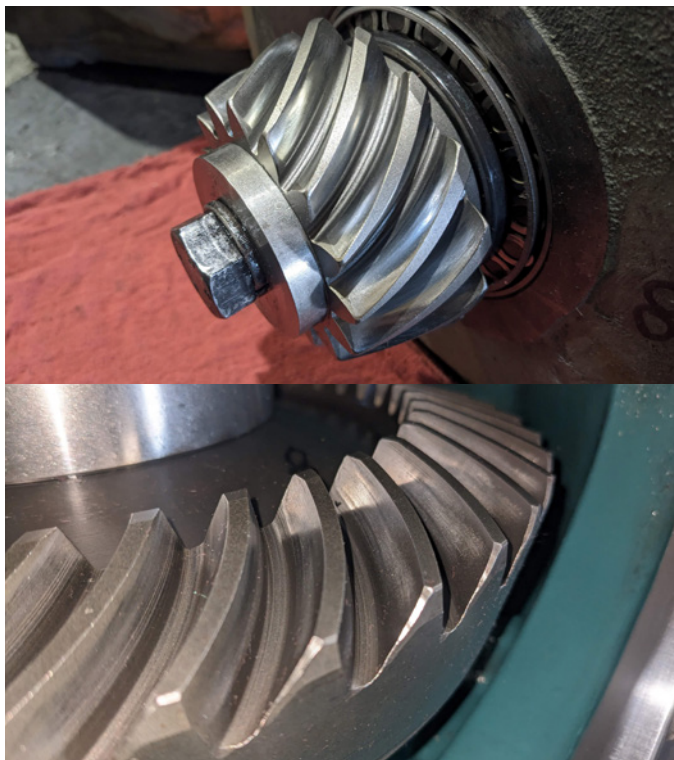
Figure 10—Bevel gear set condition. Bevel pinion shows mild polishing (top), and bevel gear shows mild polishing (bottom).
