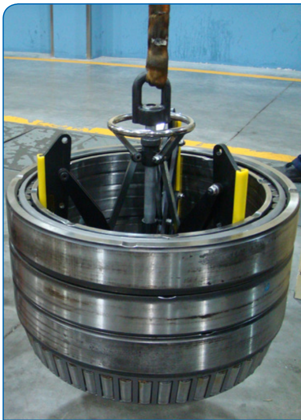
Figure 2 A three-legged (left) and sliding-foot fixture (right) for lifting complete bearing assemblies.
