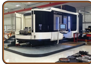
▲ DMG DMC 160 FD duoBlock® 5 axis vertical mill-turn
