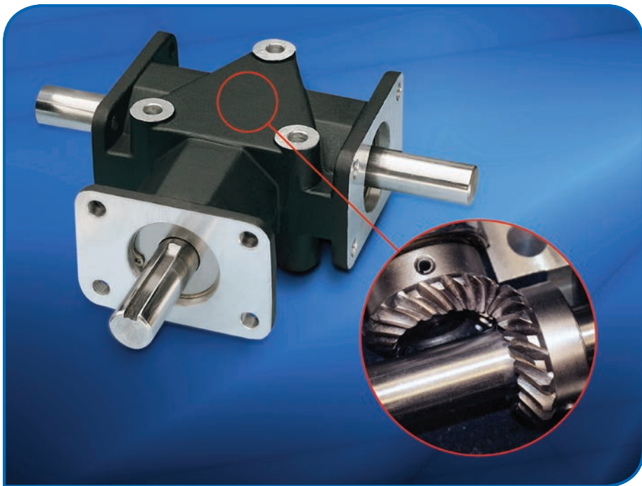
Zero-Max Crown Drives have heat treated AGMA Class 10 spiral bevel gears that are lubricated for life.
