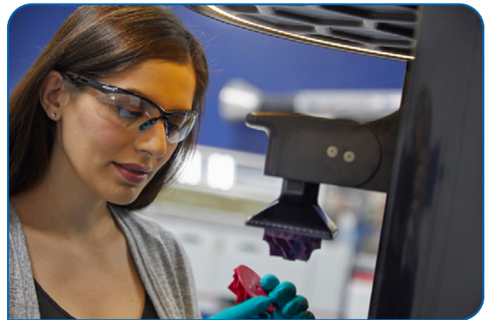
An engineer inspects a urethane methacrylate (UMA) impeller that was 3D printed using digital light synthesis (DLS) technology. Courtesy of Eaton.
