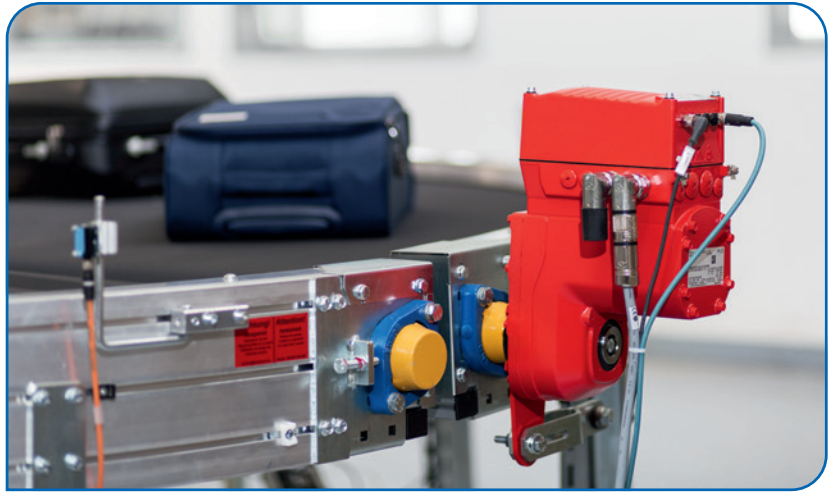
Decentralized control can include add-on components mounted on or near the motor. This modular installation can include onboard variable-frequency drives (VFDs), I/O ports, and various fieldbus options. (Image courtesy SEW-Eurodrive)
