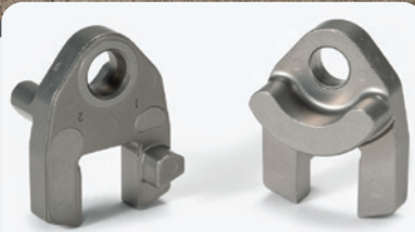
Metal Injection Molded Vane Lever used in a Turbocharger flow controller in an internal combustion engine. Typical operating temperature is 850 °C.
