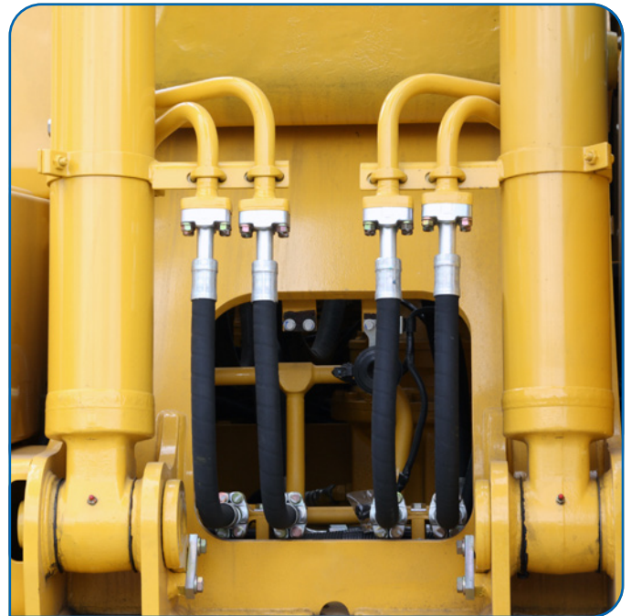
Hydraulic hoses of a modern tractor.
