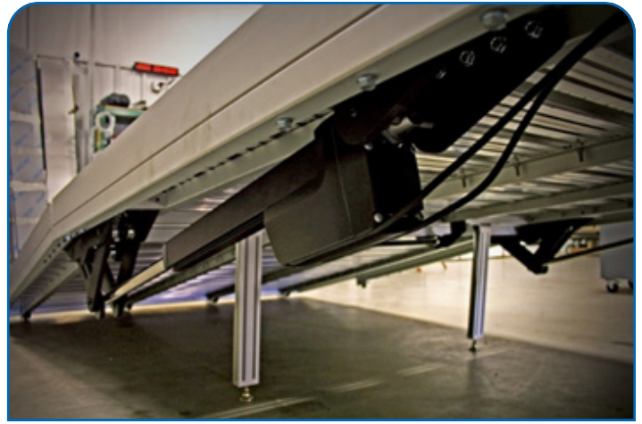
Figure 2 Four Thomson Electrak HD electric actuators (two on the floor and two below the ramp) allow The Clubhouse to safely control trailer ramp movement.
