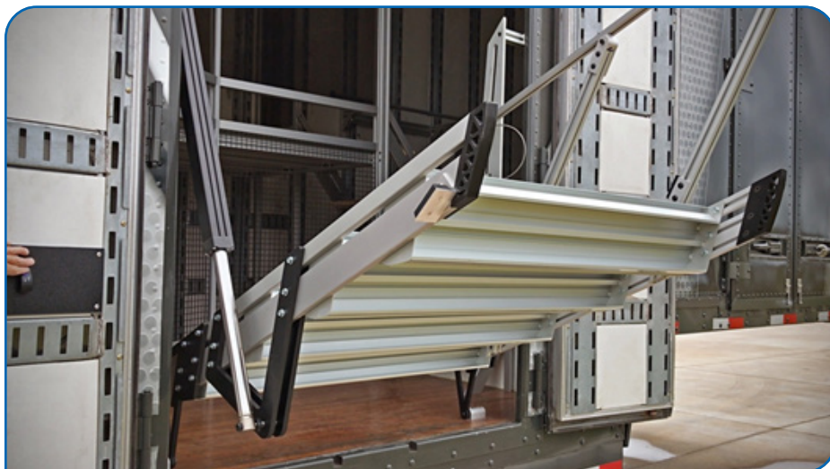
Figure 5 Electric-driven stairs have opened up new, safer accessibility options for The Clubhouse trailers.
