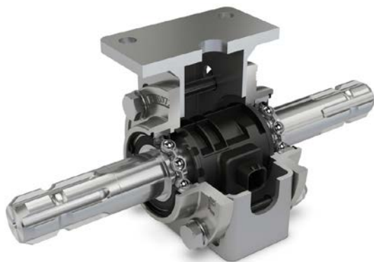
This FAG torque measurement module for agricultural applications transfers its data to the control system via the ISOBUS. All relevant parameters such as the speed and torque of the take-off shaft, the push-off speed, and the system's hydraulic pressure are recorded using sensors and then processed in the control unit.
