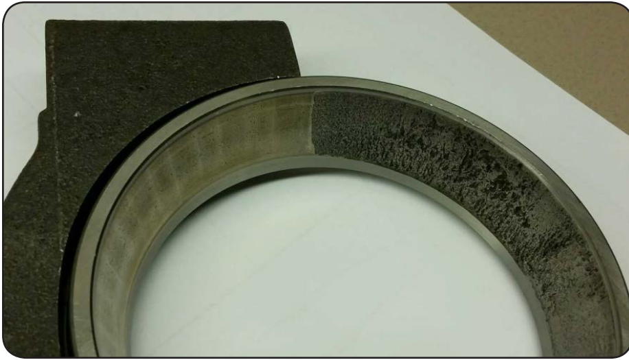
Figure 3 Bearing cup spalling at the cap interface.
