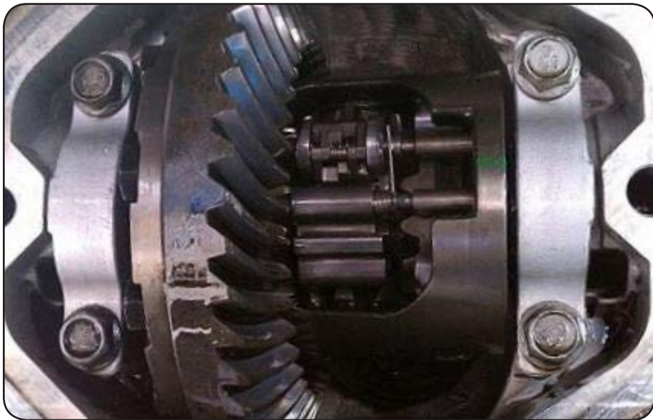
Figure 1 Rear-view Salisbury-style axle.
