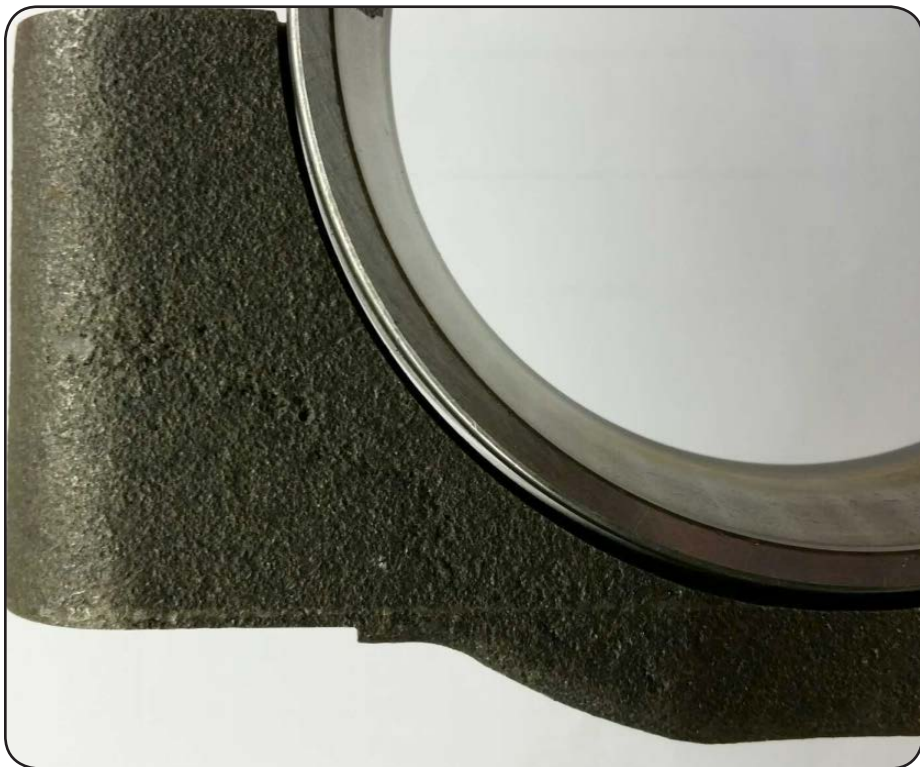
Figure 2 Bearing cap after machining and removal.
