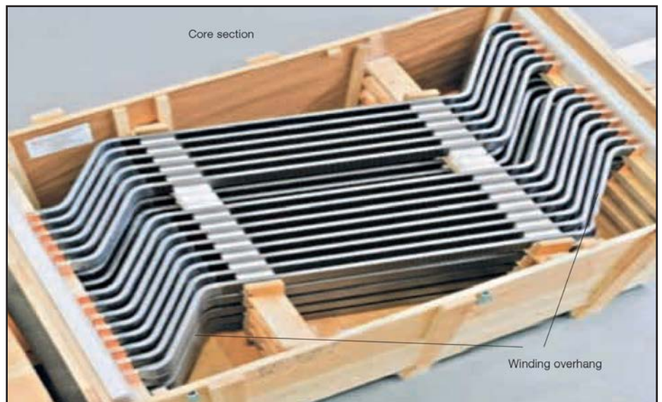
Figure 6 Full vacuum pressure impregnation for windings.
