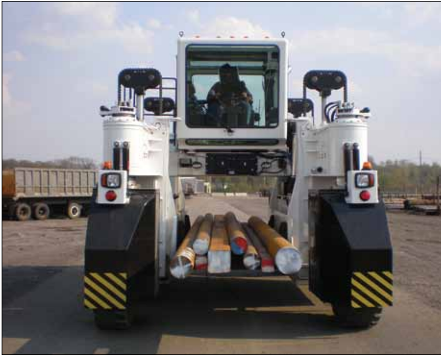
Because the straddle carrier has a lifting capacity in excess of its own empty weight, the brake system must have the ability to modulate the braking pressure.
