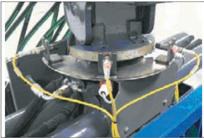
Figure 9—Sensor configuration for determining boom rotation.
