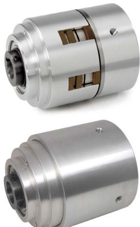
In dusty environments, Mach III offers a cover modification by increasing the outside diameter of the cylinder and machining it to cover the open portion of the clutch-brake.
