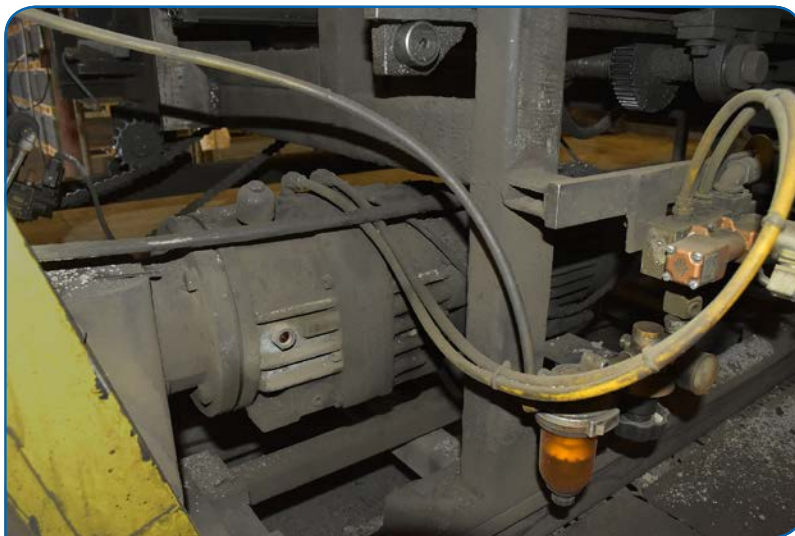
Clutch brake on main conveyor line.
