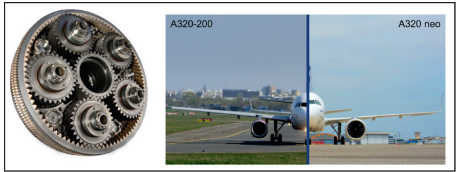
Figure 6 Geared turbofan — planetary gear stage (left) and comparison of Airbus A320-200 and Airbus A320 neo (right). (Left image courtesy of Pratt & Whitney, Right image courtesy of Airbus).
