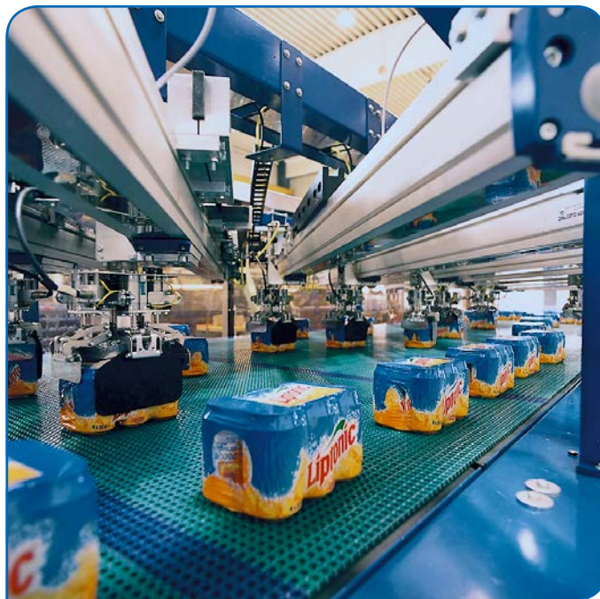
Rodless actuators are highly used in packaging application machines as they provide efficient and precise load handling solutions.
