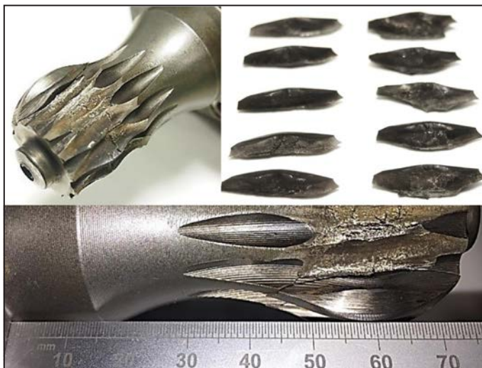
Figure 8 Teeth failure of the experimentally tested spherical gear couplings due to bending fatigue.
