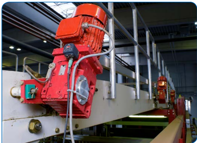
Smart technology can be used on a single machine or on a larger system of machines, including the equipment that connects those machines, like conveyors and robots. In its gray casing, a sensor monitors the operation of a motor for a conveyor belt. (Photo courtesy of Schaeffler Group USA Inc.)
