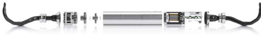
The active roll control system compensates movements in an automobile chassis caused by driving around corners or on uneven road surfaces.
