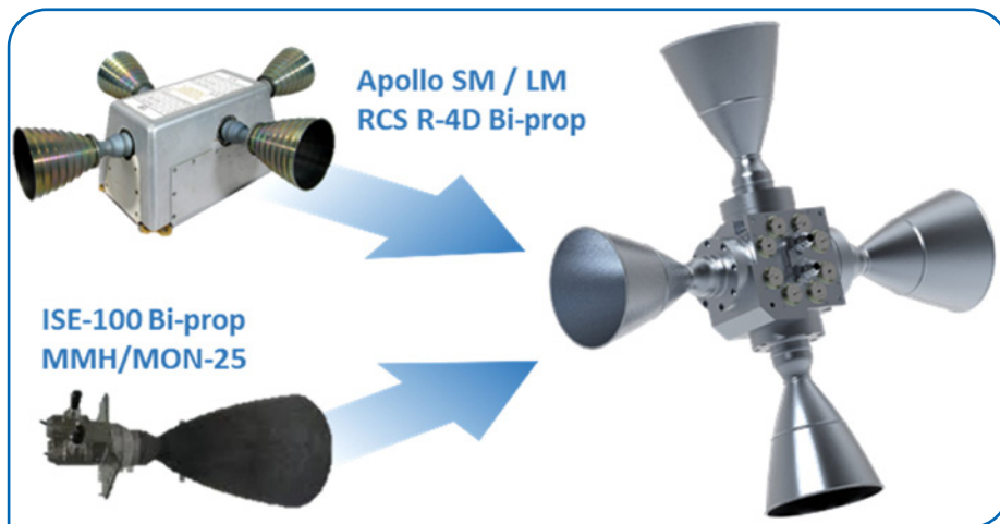
Even the first 3D-printed version of the revamped R-4D reaction control system was a huge improvement over its predecessor. AM technology from Velo3D made it even better.
