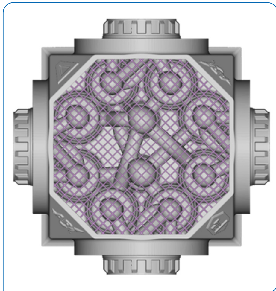
nTopology’s implicit modeling function was able to quickly “shell and fill” the injector body’s first design iteration, increasing its strength and printability while greatly reducing weight.
