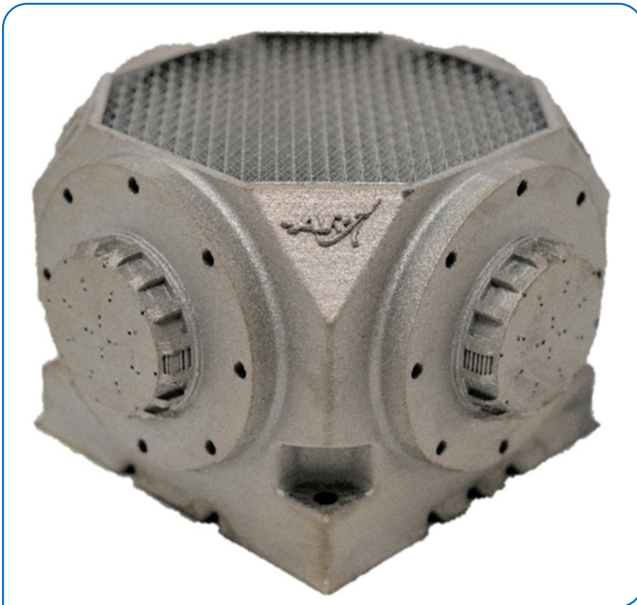
The final version of Aerojet Rocketdyne's “Mk. II” RCS injector block, shown in its as-built orientation.
